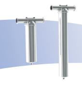
The Binks range of cartridge filters remove dirt and paint clots from paint systems using a choice of disposable or cleanable filters elements. They allow the rapid replacement of the elements with their "fixed in place" clamp design. The housing also provides an integral pressure gauge port to allow for the measurement of differential fluid pressure.
