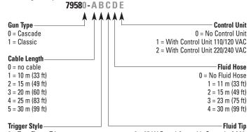
2 = Two-Finger Trigger 4 = Four-Finger Trigger 0 = 85 kV Barrel Assembly, Cascade AA90, 0811 Carbide Tip without preorifice 1 = 85 kV Barrel Assembly, Cascade AA90, 0813 Carbide Tip without preorifice 2 = 85 kV Barrel Assembly, Cascade AA90,
