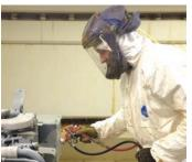
flow of compressed air through the gun body. This "free breathing" air movement enables the precisionengineered air caps and fluid tips to produce superior atomisation with consistent even distribution throughout the spray pattern. Advance HD is precision built using the best materials and component parts for a guaranteed, reliable, long and durable working life in all industrial markets.
